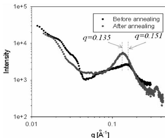
Fig. 4. SAXS of the composite membranes containing EMIBF<sub>4</sub> before and after annealing at 190 °C for 2 h.
