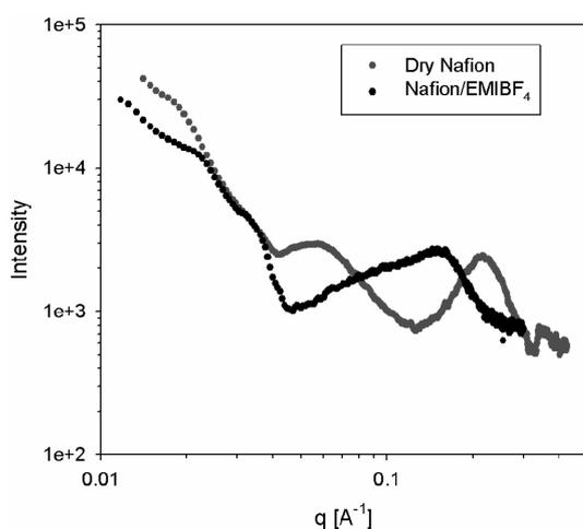
Fig. 3. SAXS of the Nafion recast membranes and the composite ones containing EMIBF<sub>4</sub>.
