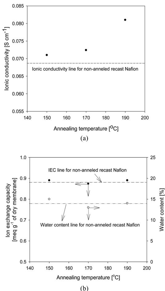
Fig. 1. (a) Variation of ionic conductivity (at fully hydrated status and room temperature) (b) variation of ion exchange capacity (IEC) and water content with annealing temperature for recast Nafion membranes.
