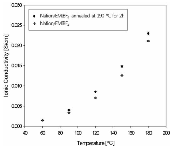
Fig. 2. Variation of ionic conductivity (under anhydrous status) with temperature for the composite membranes containing EMIBF<sub>4</sub> before and after annealing at 190 °C for 2 h.
