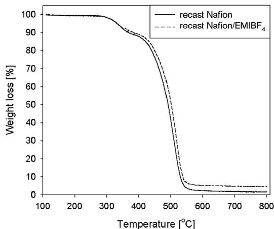
Fig. 6. Thermogravimetric analysis curves of recast Nafion and composite membranes containing EMIBF<sub>4</sub> under nitrogen atmosphere.
