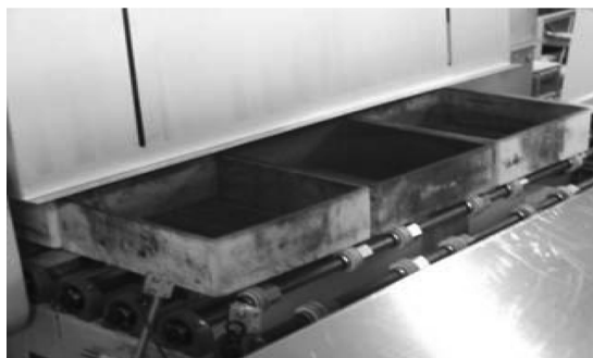
Fig. 5. Calcination furnace to produce cathode active materials.
