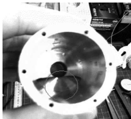
Fig. 6. Photo of condensed water in the outer conductor during the DMFC test with an open-type flow field.
