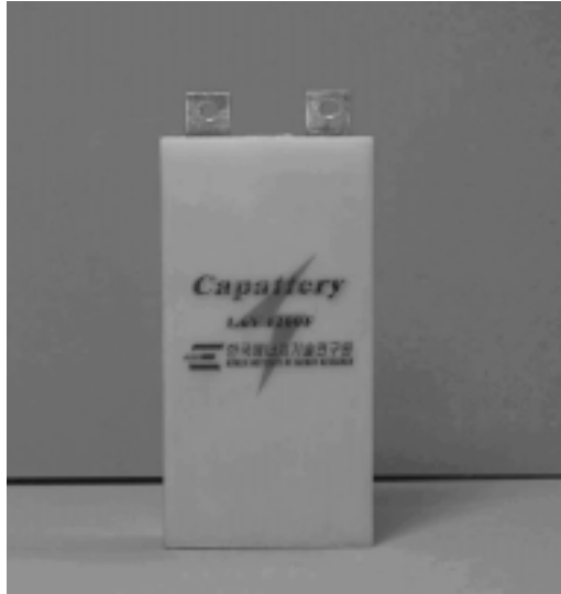
Fig. 8. Photo of a proto-type hybrid capacitor.
