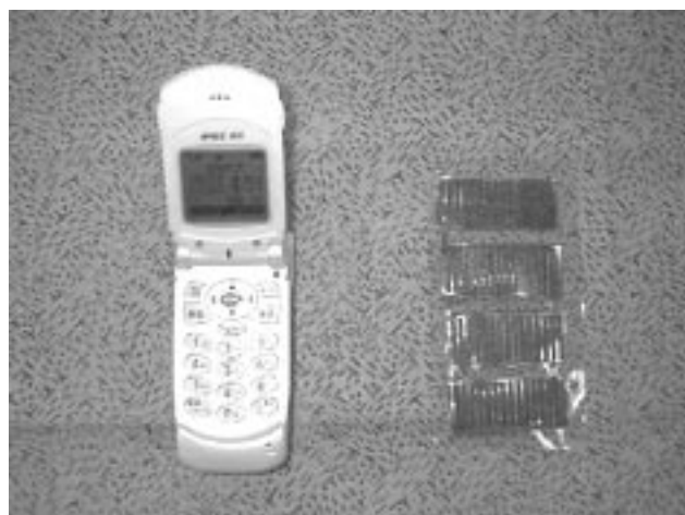
Fig. 1. Photograph of monopolar containing four MEA connected in series.
