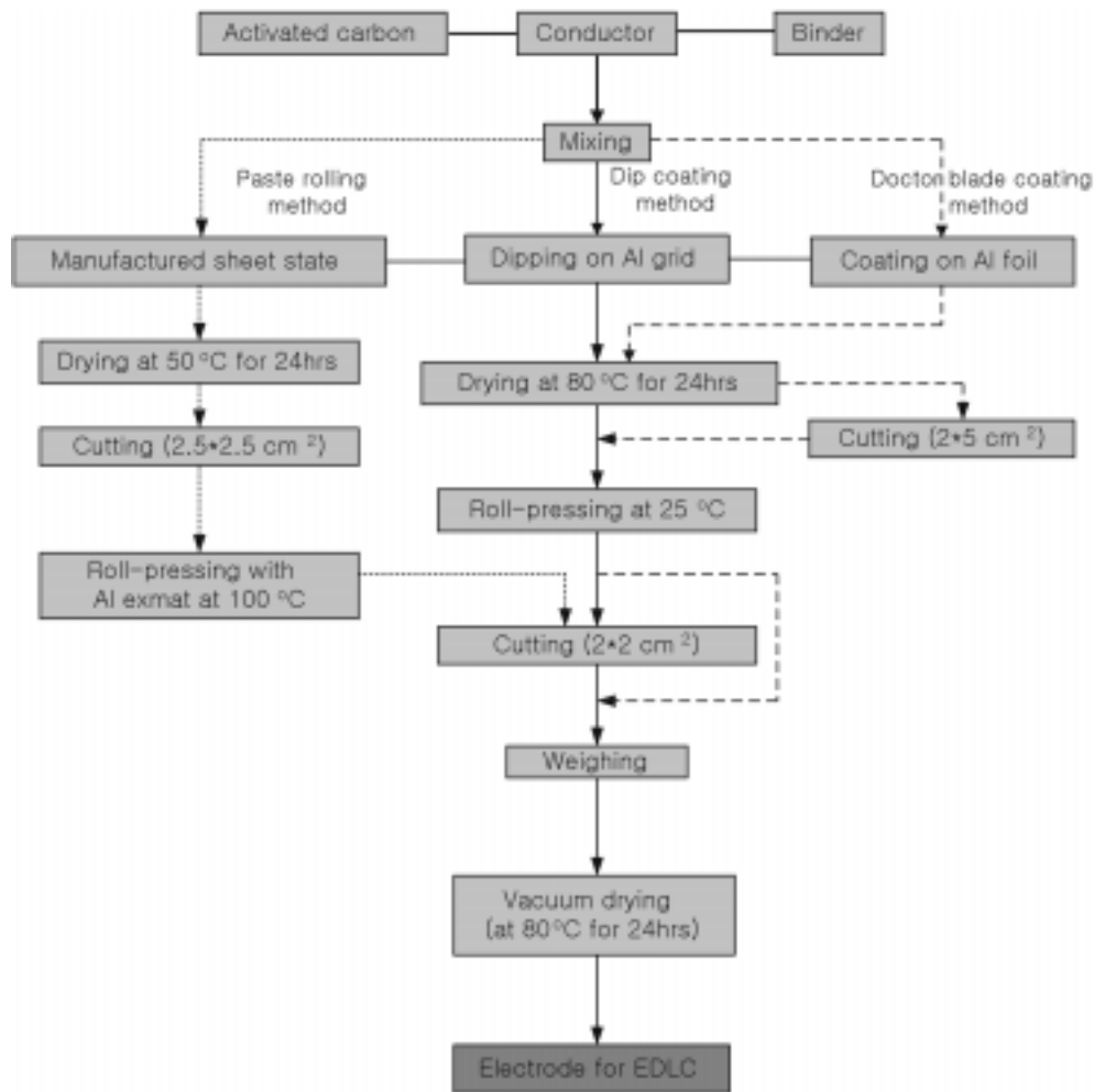
Fig. 1. Procedure of various preparation method of electrode for EDLC.
