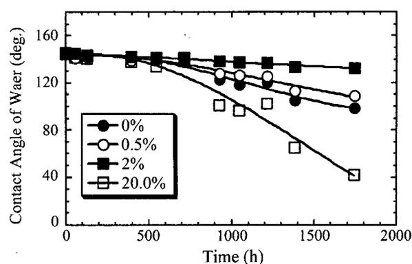
Fig. 5. The effect of  $\text{TiO}_2$  addition on the water contact angle during outdoor exposure.
