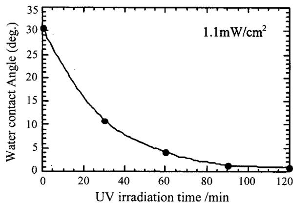
Fig. 3. Effect of UV irradiation on water contact angle.
