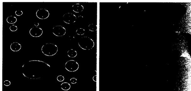
Fig. 2. Change in shape of water droplets after irradiation.
