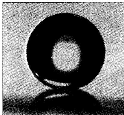
Fig. 4. The shape of water droplet on the super-hydrophobic film.
