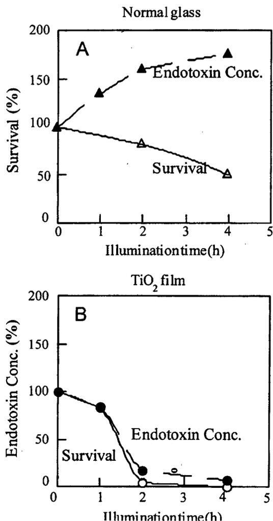
Fig. 1. Concentration change of the endotoxin exhausted from *E. coli* and survival ratio of *E. coli* under UV light illumination ( $0.4 \text{ mW/cm}^2$ ) on TiO<sub>2</sub> coated glass and normal glass.
