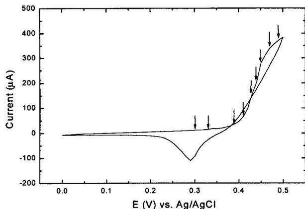
Fig. 5. Cyclic voltammogram for oxidation of 0.20 M ethanol at a RuO<sub>2</sub>-modified nickel electrode (0.17 cm<sup>2</sup>) in 1 M KOH at 10 mV/s. Impedance measurements were made at potentials marked.
