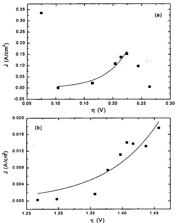
Fig. 7. (a) The current density vs. overpotential for  $R_1$  for oxidation of 0.20 M ethanol in 1 M KOH. The line drawn is from the nonlinear least squares fitting for the data between 0.33 and 0.45 V; (b) Current density vs. overpotential for  $R_2$ . The nonlinear least squares curve fitting is drawn for the data obtained between 0.30 and 0.49 V.
