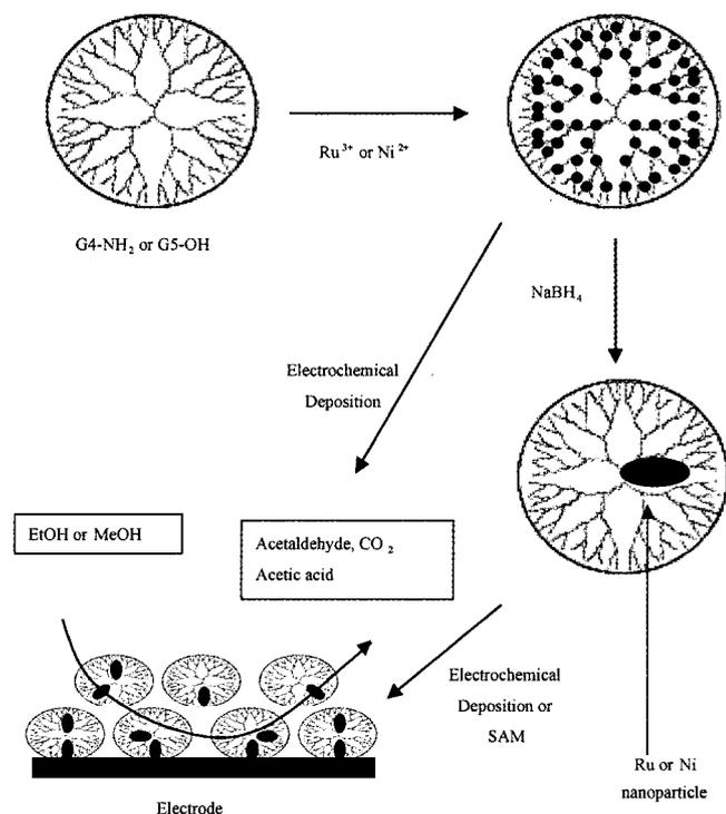
Fig. 1. Schematic diagram for the preparation of nanoparticles by electrochemical deposition and/or chemical reduction of Ru, Ni, or Ru-Ni ions complexed within G4(NH<sub>2</sub>) and/or G5(OH) PAMAM dendrimers.
