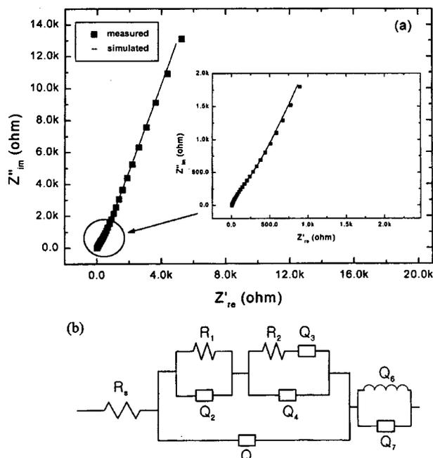
Fig. 3. (a) Complex impedance responses for oxidation of the  $\text{RuO}_2$ -modified nickel electrode at 0.32 V in 1 M KOH; (b) an equivalent circuit used in the CNLS fitting procedure.
