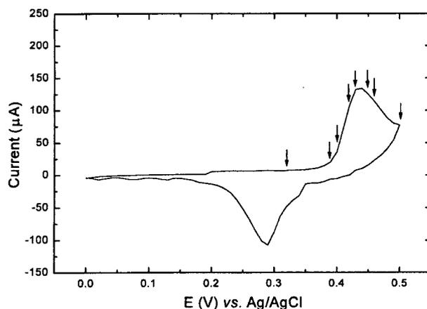
Fig. 2. Cyclic voltammogram of a RuO<sub>2</sub>-modified nickel electrode (0.17 cm<sup>2</sup>) in 1 M KOH at 10 mV/s. Impedance measurements were made at potentials marked.
