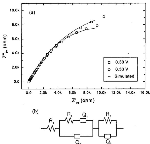
Fig. 6. (a) Complex impedance responses for oxidation of ethanol at RuO<sub>2</sub>-modified nickel electrode at 0.30 and 0.33 V in 1 M KOH containing 0.20 M ethanol; and (b) An equivalent circuit used in the CNLS fitting procedure.
