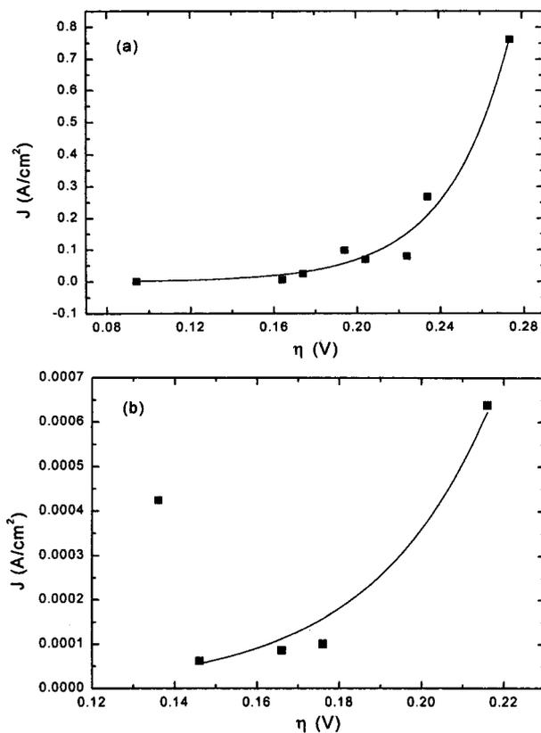
Fig. 4. (a) Current density calculated from  $R_1 + R_2$  vs. overpotential in 1 M KOH. The line drawn is from nonlinear least squares (NLS) fitting using Butler-Volmer equation for the data between 0.32 and 0.50 V; (b) current density vs. overpotential for  $R_3$  in 1 M KOH with the NLS line drawn for the data between 0.42 and 0.50 V.
