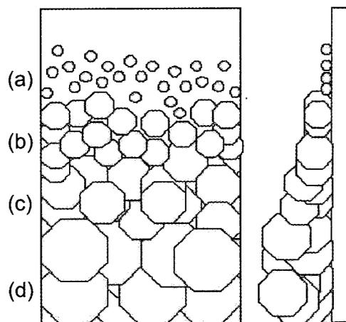
Fig. 2. Schematic diagram of diamond film which deposited on inclined substrate.
