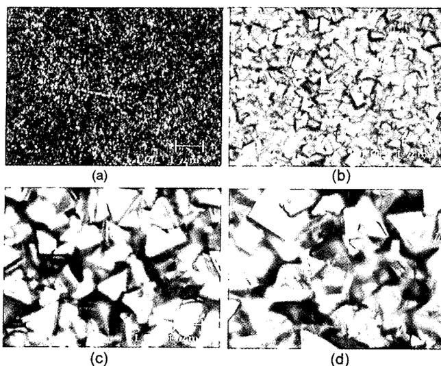
Fig. 5. Microscope images of diamond film, which deposited for 3 hrs on Si wafer. (Magnified 2500 times); (a) : 750°C, (b) : 820°C, (c) : 860°C, (d) : 980°C.
