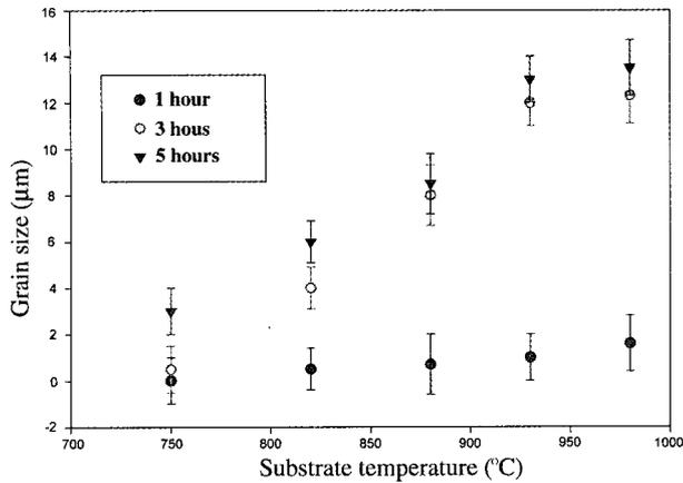
Fig. 9 Relationship between temperature and grain size.
