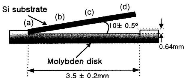
Fig. 1. Schematic Specimen setting for inclined substrate.
