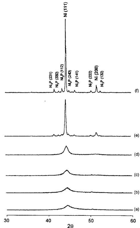
Fig. 4. X-ray diffraction of deposits for heating temperature. (a)As deposited, (b) 200°C, (c) 300°C, (d) 400 °C, (e) 500°C, (f) 600°C
