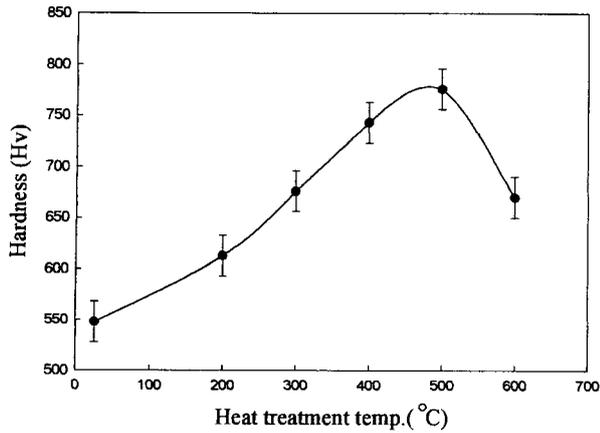
Fig. 3. Effect of heat treating temperature on hardness of electroless nickel deposits. (hardness of copper substrate : 140 Hv)
