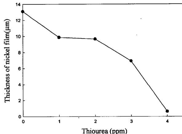
Fig. 2. Thickness variation of nickel film with concentration of thiourea.
