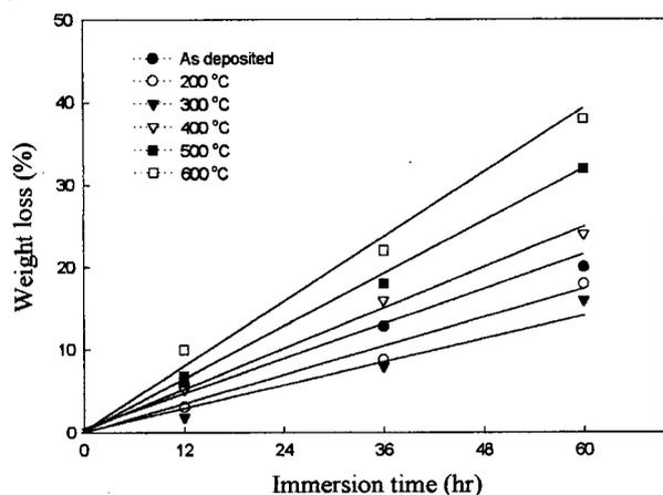
Fig. 6. Weight loss of electroless nickel film at 1 M H<sub>2</sub>SO<sub>4</sub> solution.
