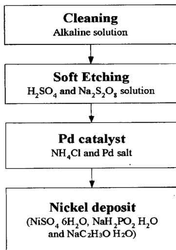
Fig. 1. Flow chart of Electroless Ni-P plating process.
